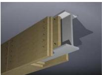
As to the beam lining, prepare fixing plates of Grenamat AL boards being 12 mm thick, 150 mm wide. Define the length according to the particular length of the beam to be lined (Fig.). Join the two 12 mm thick fixing plates using at least 4 clips. Use 30-50mm long and at least 10 mm wide clips.
